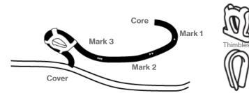
To splice into a thimble with ears, shackle, or similar item, simply follow the directions of the splicing instructions, using the thimble or shackle bale to determine the eye size. Extract the core and insert the core through the bale or around the shackle as illustrated. The eye splice is then completed in a normal fashion with one exception: before final bury, slide the thimble around to cover side of eye. For a thimble without ears: insert thimble into eye before final burying of splice.
