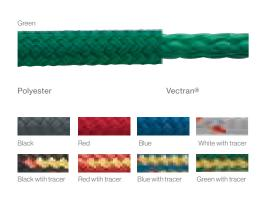
The ultimate in high load performance, V-100 features a braided 100% Vectran<sup>®</sup> 12-strand single braid core treated with our unique marine-tech coating with a highly durable and attractive polyester cover. V-100 is a very strong, low stretch, high-tech line for its size and it has good abrasion resistance and virtually no creep.
